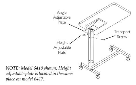
FIGURE 3 Operating the Overbed Table - Adjusting Table Height - Adjusting Table Angle - Model 6418 ONLY
